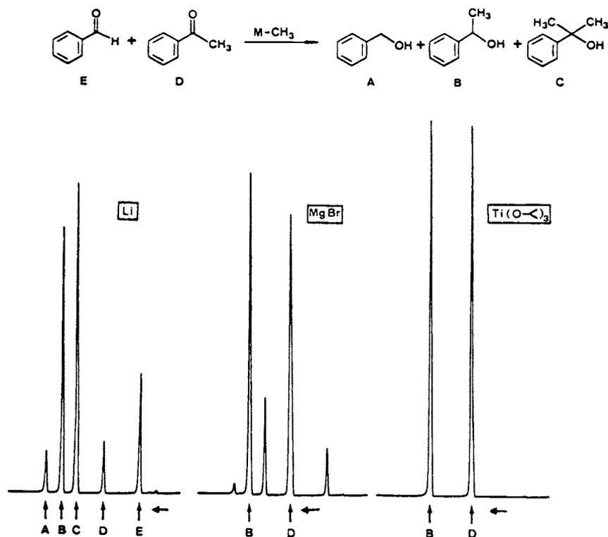
Fig. 1: Mixtures obtained from methyl-metal derivatives and a 1:1-mixture of  $C_6H_5CHO$  and  $C_6H_5COCH_3$  at room temperature (see also ref.<sup>1,2</sup> and accompanying text).
