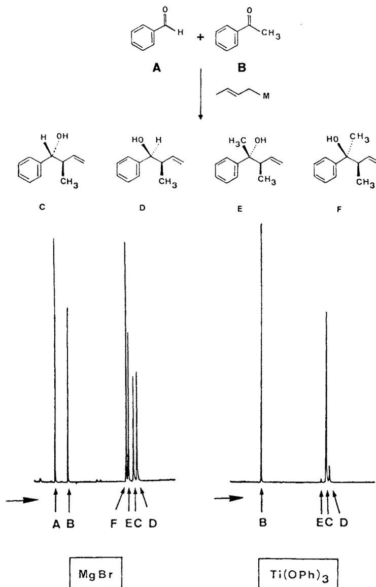
Fig. 2: GC-chromatograms obtained after reaction of crotyl-magnesium bromide and of crotyl-triphenoxy-titanium with a 1:1-mixture of benzaldehyde and acetophenone.<sup>10</sup>
